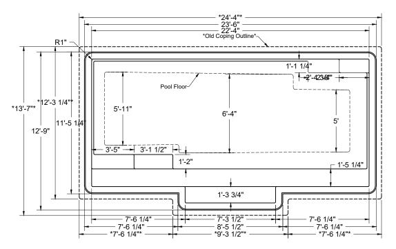
Length, width and depth may vary up to 3% - all dimensions are to outside edge of coping, measured from parallel lines. All other dimensions +/- 1inch.
